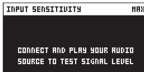
Sets the audio input level to fit the audio level sent to the effect via the IN L/R inputs. It is important to set this level correctly to get the best sound from your Analog Heat +FX. There are four different settings for the input sensitivity: LOW, MID, HIGH & MAX. Low is the most silent, Max is the loudest. For more information, please see "3.2 SETTING THE INPUT SENSITIVITY LEVEL" on page 10.
