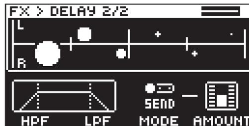
**HPF** Sets the cutoff frequency of the delay highpass filter.
