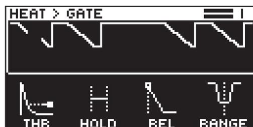
**THRESHOLD** Sets the audio input level at which the gate will open and let through a signal.
