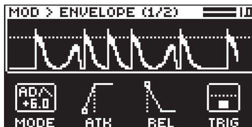
9. Press the **[MOD]** key, navigate to ENVELOPE page 2 and change **DEST1** to PST VOLUME and **DEPTH1** to -72.
