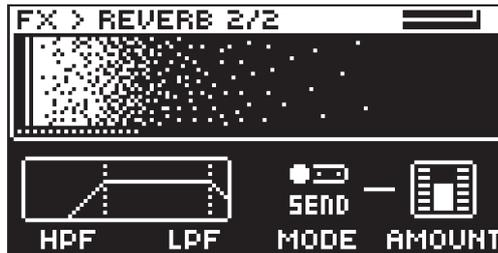
**HPF** Sets the cutoff frequency of the reverb highpass filter.
