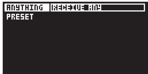
The column to the left selects what will be received. Use the **NAVIGATION** knob to navigate in the column. The SysEx data receive alternatives located in the column to the right will change depending on the selection made in the left column. Press **[YES]** to access this column. Use the **NAVIGATION** knob to select what will be received. Press **[YES]** to initiate the SysEx receive procedure. The Analog Heat +FX starts listening to incoming data. Press **[NO]** to stop listening.
